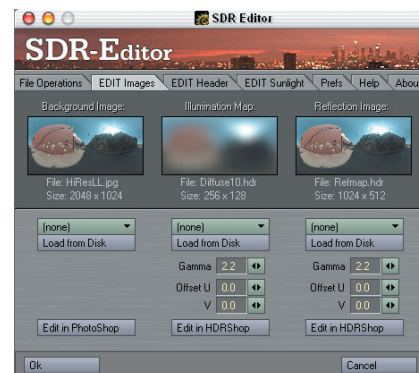
Figure 3: SDR Editor prototype, a tool for lighting TDs. Pictured are the 3 images that are bundled in a SDR preset.
